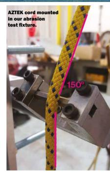
still non-standardized abrasion test. With the Aramid AZTEK kit in mind, the Sterling Engineering Team gathered knowledge from past and applicable attempts to solve this problem and modified our cycle test stand to accept a new abrasion test method.
