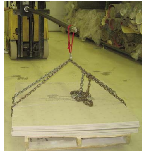
Preloading individual nylon slings to 500 lbs in order to decrease knot slippage during strength testing
