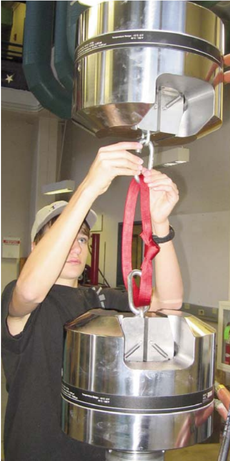
Photo shows jaws of Material Testing System (MTS) 810 clamping chain link with webbing being attached to Mailons to be pulled until failure
