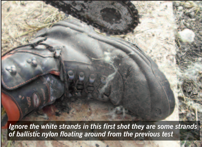
First Hit, through leather and Kevlar layer 1, stalled at Kevlar layer 2. This looks like ballistic nylon but is strands from a double thickness sheet.
