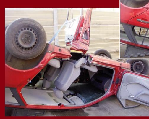
The base of the B pillar can be large and require several cuts if you need to remove the side completely. Alternatively you can take advantage of the space above the vehicle to leave the pillar attached and fold it up above and out of the way.
