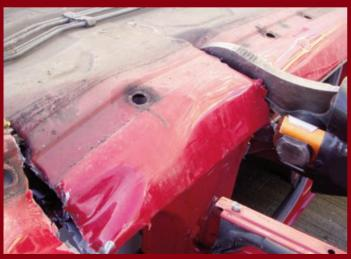
Then make a further deep relief cut again at 90 degrees to the sill immediately in front of the B pillar again ensuring the cut is completely through the sill.
