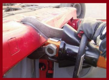
Make a deep relief cut in the sill at 90 degrees immediately behind the B pillar ensuring you cut through the sill completely.
