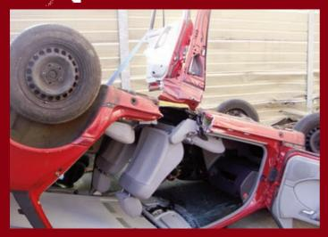
Then fold it up above and out of the way and secure with a ratchet strap
